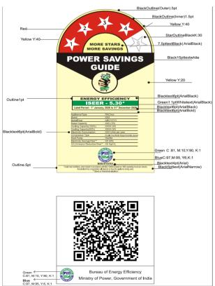
(iii) The complete specimen of a printed label for room air conditioner;
